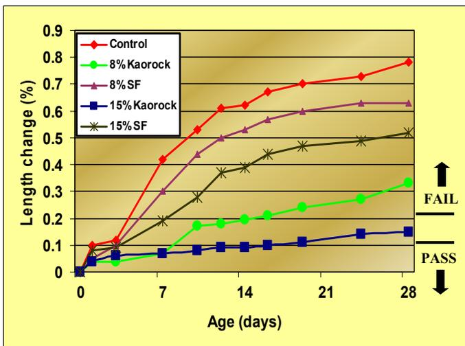
Figure 3: Expansion due to alkali-silica reaction, w/cm = 0.47, was measured according to the accelerated mortar bar method (ASTM C 1260). This method has proven reliable for evaluating the effectiveness of SCM's in suppressing ASR. KAOROCK™ passed while the control and samples made with silica fume failed.
