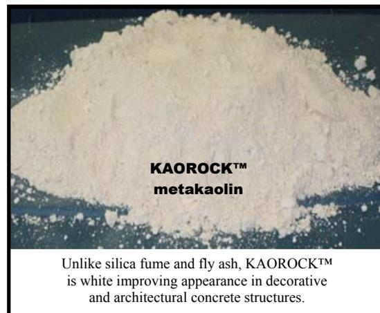
KAOROCK™ is a metakaolin that enhances the properties of concrete and cement-based products. It is an ultra-fine material that is white in color produced from kaolin, an aluminum silicate mineral mined in middle-Georgia. Because KAOROCK™ is not a by-product as other pozzolans on the market such as silica fume and fly ash, product quality and specifications can be strictly controlled from batch to batch.
